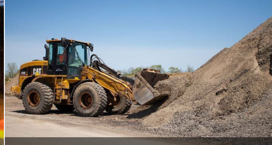
Recycled asphalt grindings used for shoulder repairs
