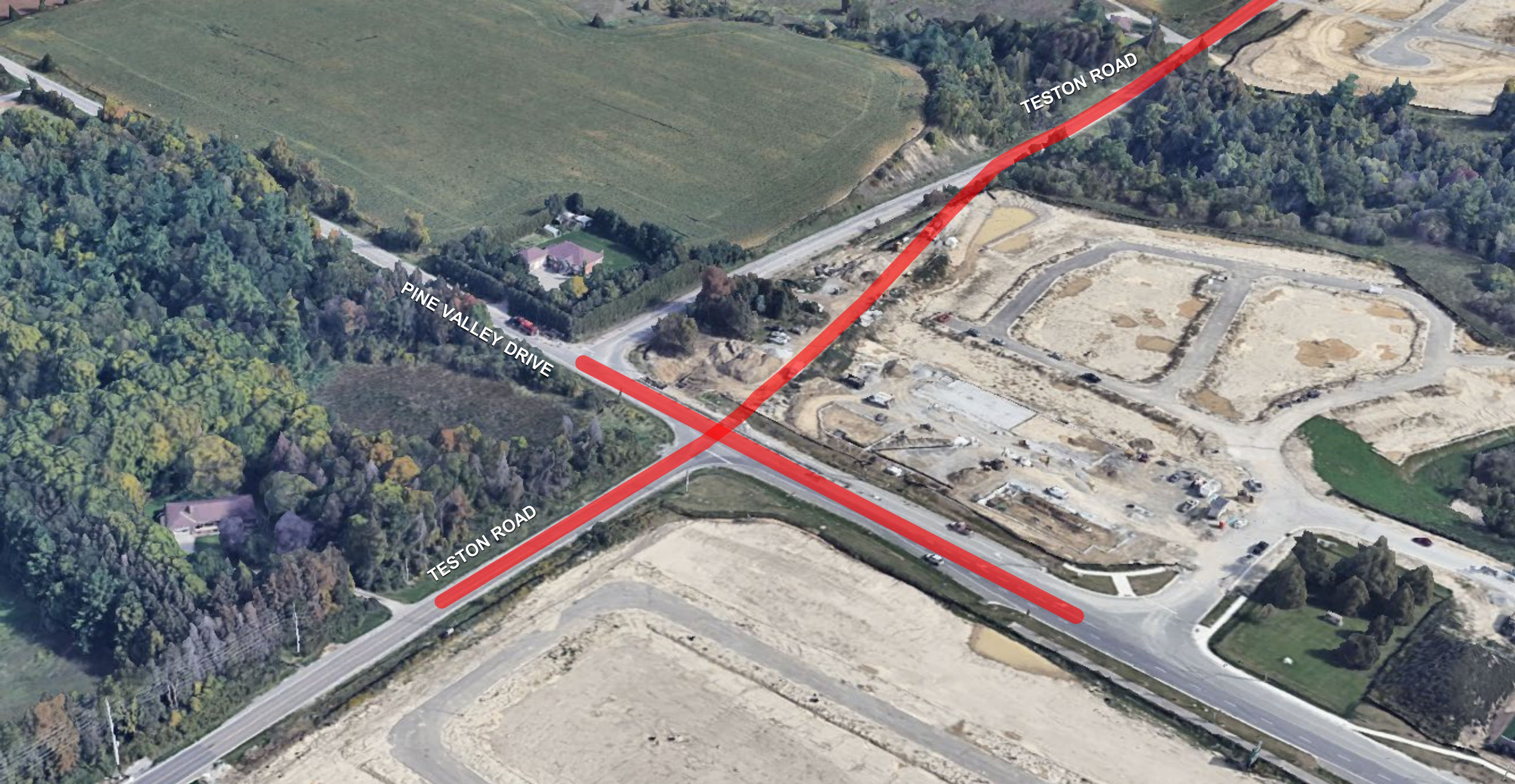
Road widening from two to four lanes, including a jog elimination and new traffic signals at Pine Valley Drive
