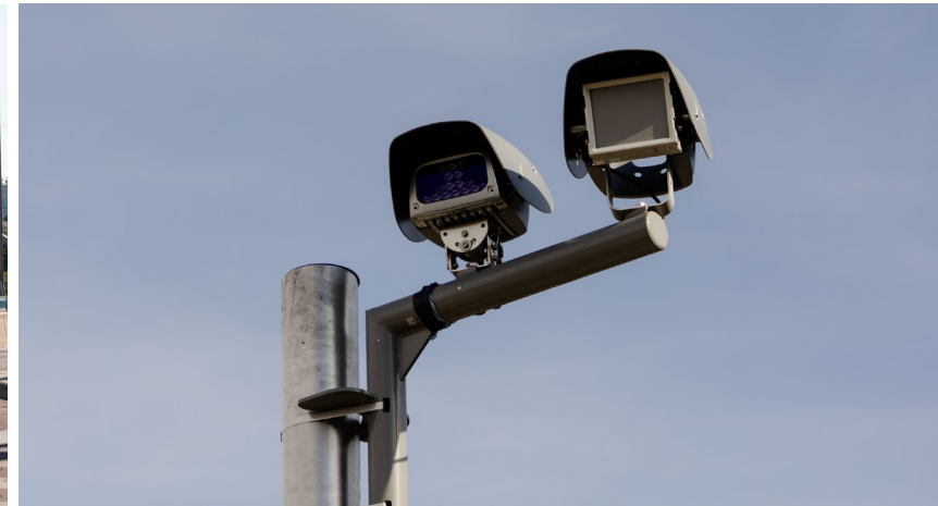
Automated Speed Enforcement Camera, Town of East Gwillimbury
