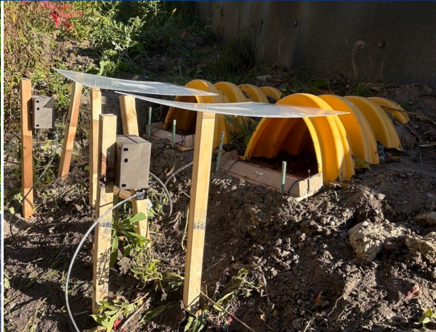
Infrared cameras at new wildlife crossing on Stouffville Road, City of Richmond Hill
