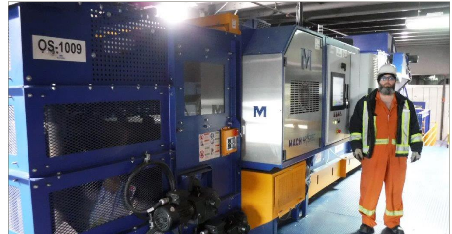
Optical Sorter improves overall quality of fibre and plastic bales
